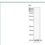
Western blot testing of human HepG2 cell lysate with UFM1 antibody. Predicted molecular weight: 9-11 kDa (two isoforms).
