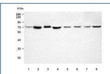
Western blot testing of 1) human T-47D, 2) human MDA-MB-453, 3) PC-3, 4) MCF7, 5) rat brain, 6) rat PC-12, 7) mouse brain and 8) mouse RAW264.7 cell lysate with TMEM87A antibody. Predicted molecular weight ~63 kDa but may be observed at higher molecular weights due to glycosylation.
