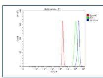
Flow cytometry testing of human 293T cells with SEC22B antibody at 1ug/million cells (blocked with goat sera); Red=cells alone, Green=isotype control, Blue= SEC22B antibody.
