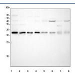
Western blot testing of 1) human U-87 MG, 2) human HeLa, 3) human MCF7, 4) human SH-SY5Y, 5) rat brain, 6) rat liver, 7) mouse brain and 8) mouse liver tissue lysate with SEC22B antibody. Predicted molecular weight ~25 kDa.
