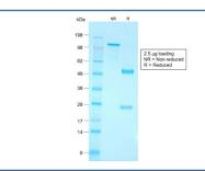
SDS-PAGE analysis of purified, BSA-free recombinant CD79a antibody (clone IGA/1790R) as confirmation of integrity and purity.
