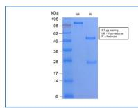
SDS-PAGE analysis of purified, BSA-free recombinant CD68 antibody (clone C68/2908R) as confirmation of integrity and purity.
