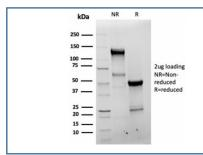
SDS-PAGE analysis of purified, BSA-free recombinant Bcl-X antibody (clone BCL2L1/4509R) as confirmation of integrity and purity.
