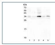
Western blot testing of 1) rat thymus, 2) rat kidney, 3) rat testis, 4) mouse kidney and 5) mouse testis lysate with PPA1 antibody at 0.5 ug/ml. Predicted molecular weight:  $\sim 33 \text{ kDa}$ .
