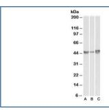
Western blot of A549 (A), HepG2 (B) and HeLa (C) lysates with PAI-1 antibody at 0.1ug/ml. Predicted molecular weight ~45kDa.
