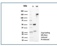
SDS-PAGE analysis of purified, BSA-free NTRK2 antibody (clone NTRK2/4672) as confirmation of integrity and purity.
