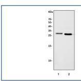
Western blot testing of 1) rat liver and 2) mouse liver tissue lysate with Nr0b2 antibody. Predicted molecular weight ~28 kDa.
