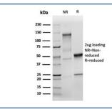
SDS-PAGE analysis of purified, BSA-free MSH2 antibody (clone MSH2/6549R) as confirmation of integrity and purity.
