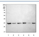
Western blot testing of 1) human HepG2, 2) human SH-SY5Y, 3) human MCF7, 4) rat C6, 5) mouse brain and 6) mouse Neuro-2a cell lysate with LRRC75B antibody. Predicted molecular weight ~35 kDa.
