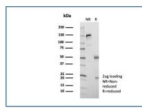
SDS-PAGE analysis of purified, BSA-free Kinesin-like protein 6 antibody (clone KIF2C/6524) as confirmation of integrity and purity.
