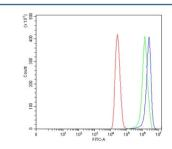
Flow cytometry testing of human MCF7 cells with JUP antibody at 1ug/million cells (blocked with goat sera); Red=cells alone, Green=isotype control, Blue= JUP antibody.
