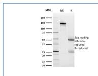
SDS-PAGE analysis of purified, BSA-free HER2 antibody (clone ERBB2/2453) as confirmation of integrity and purity.
