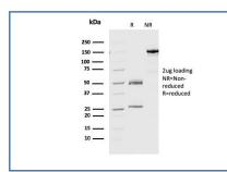
SDS-PAGE analysis of purified, BSA-free Geminin antibody (clone CPTC-GMNN-1) as confirmation of integrity and purity.
