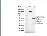
SDS-PAGE analysis of purified, BSA-free FXN antibody (clone FXN/2124) as confirmation of integrity and purity.
