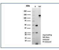
SDS-PAGE analysis of purified, BSA-free ERCC1 antibody (clone ERCC1/7596) as confirmation of integrity and purity.
