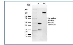
SDS-PAGE analysis of purified, BSA-free EGFR antibody (clone 225) as confirmation of integrity and purity.
