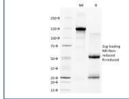
SDS-PAGE Analysis of Purified, BSA-Free CD28 Antibody (clone C28/77). Confirmation of Integrity and Purity of the Antibody.
