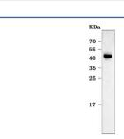
Western blot testing of human SH-SY5Y cell lysate with C12orf53 antibody. Predicted molecular weight ~30 kDa but may be observed at higher molecular weights due to glycosylation.
