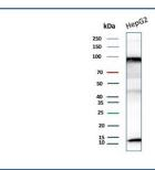
Western blot testing of human HepG2 cell lysate with BRCA1-Associated Protein 1 antibody (clone BAP1/13501R). Expected molecular weight: 80-100 kDa.
